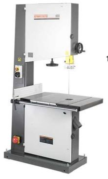
700 x 608 mm 580 mm 370 mm 1500 m/min 4470 mm 10 – 35 mm 90° - 45° 100 mm 400V/5.5 PS 330 kg 1170 x 810 x 1970 mm
